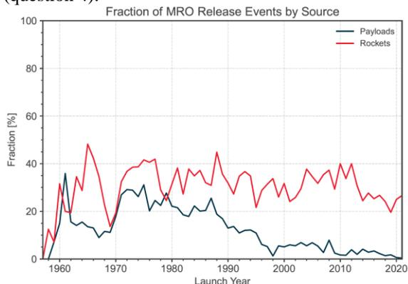
Fig. 3. Evolution of fraction of mission related objects released per year with respect to the total amount of payloads and rocket bodies injected into the space environment during that year [13].
