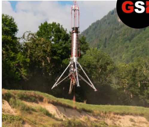
GSP's Colibri, a bi-propellant vertical take-off and landing (VTVL) rocket
