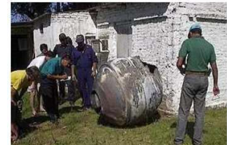
Titanium casing of the STAR-48B solid rocket motor found in northeastern Argentina.
