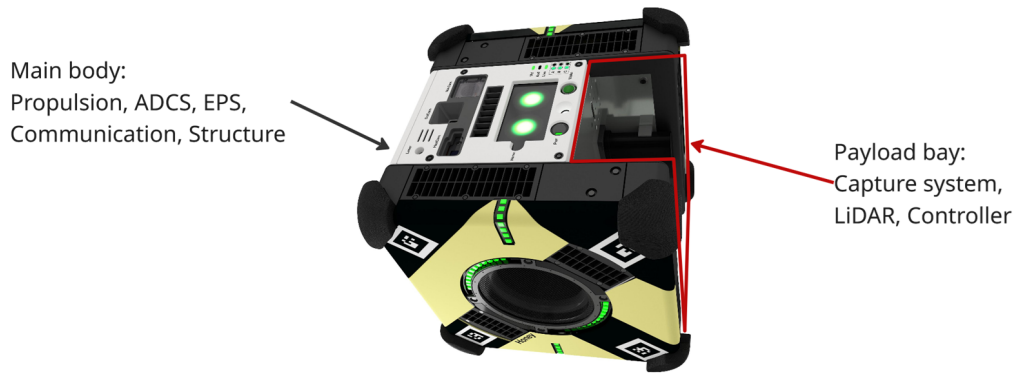
Figure 10.3: System overview of Astrobee solution (©NASA, annotated)
